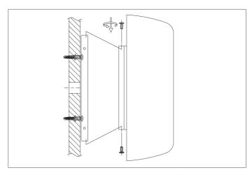
Place the lamp over the wall plate and fix it securely with the screws supplied.
