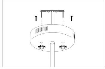
**4.** Slide the canopy over the ceiling bracket and fixt it with the two nuts.
