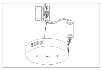
3. Connect the LED driver to the lamp according to the + and - marks. Hold the lamp in an elevated position, so the wires can reach the junction box in your ceiling. Connect the three power wires. Brown is the live wire, blue is the neutral, green/yellow is the earth wire.
