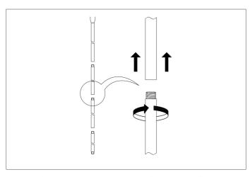
1. Determine the desired height of your chandelier and connect the extension pipes. Thread the wires through the pipes.
