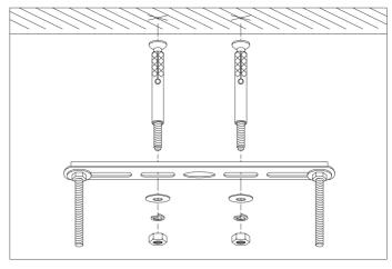
2. Fix the ceiling bracket to the ceiling by using mounting plugs and screws suitable for your ceiling type.
