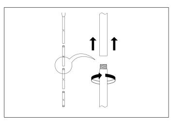
1. Determine the desired height of the lamp and use either one, two or three of the pipes supplied. Thread the wires through the pipes.
