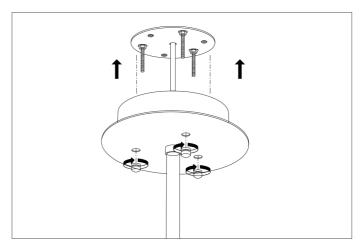
$\textbf{4.}\,\text{Place}$  the ceiling canopy over the ceiling plate and fix it securely with the three nuts.
