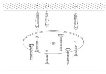
2. Fix the ceiling plate to the ceiling by using mounting plugs and screws suitable to your ceiling type
