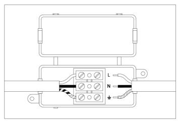
3. Connect the 3 power wires according to their colours. Brown is the live wire, blue is the neutral wire, green/yellow is the earth wire.
