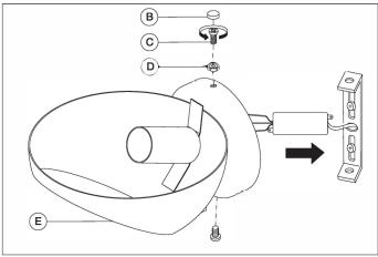
3. Place the lamp over the cross bar and alight the holes. Fix the plastic ring with the screw and cover it with the cover.
