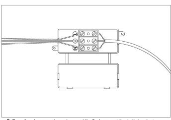
2. Open the wire connector and connect the 3 wires according to their colours . Brown is the live wire, blue is the neutral wire, green/yellow is the earth wire.
