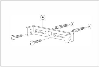
1. Fix the crossbar to the wall by using wall mounting plugs and screws uitable to your wall type.
