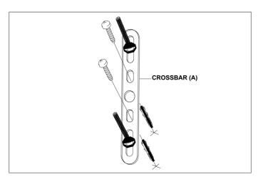
Fix the cross bar to the wall by using wall mounting plugs and screws suitable for your wall type.
