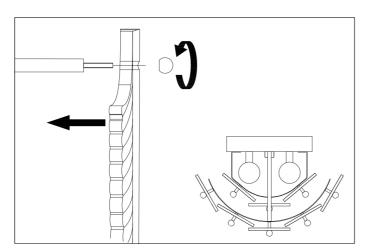
5. Place the glass pcs according to the drawing and secure them with the balls.
