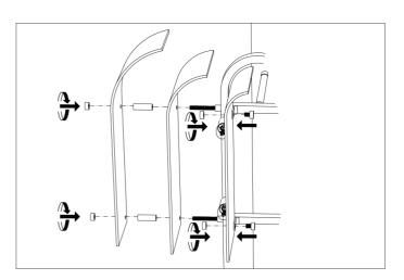
6. Place the small glass first and secure it with the nuts.
