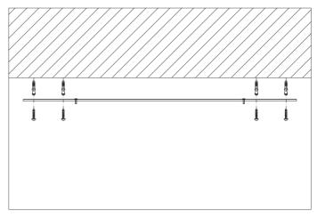
Fix the ceiling plate to the ceiling by using mounting plugs and screws suitable to your ceiling type.
