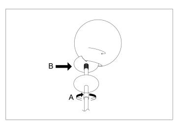
3. Tilt the glass ball so you can place it over one side of part B. Then tilt again so it is completely over part B. Now tighten part A until the glass is secure.
