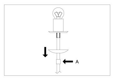
2. Unscrew the ring (part A) so you can move the cover down.
